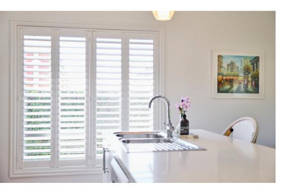
For increased strength and durability, our new generation PVC Shutters are constructed with high grade extruded Polyresin and an aluminium core in each blade and panel. Australian designed, this unique construction allows us to offer our industry leading 10 year warranty for PVC Shutters.
